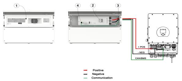
• Connection cables can exit the chassis on either left or right side, depending on the inverter location. See diagrams below for details:
