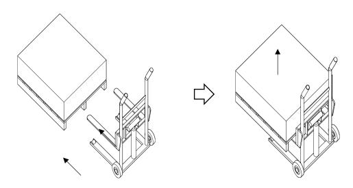
• Lift and stand battery upright onto trolley. Ensure brakes on trolley are applied.
