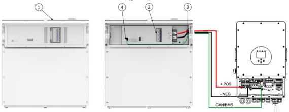
• Connection cables can exit the chassis on either left or right side, depending on the inverter location. See diagrams below for details:
