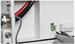
11) Connect the power cables and communication cable from the E10 (right) to inverter.
