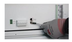
8) Connect the power cables and communication cable to the E10 on the right.
